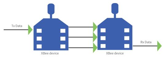
The transmit frame can include up to 255 bytes of data broken up into multiple transmissions and reassembled on the receiving side. If one or more of the fragmented messages are not received by the receiving device, it drops the entire message, and the sender indicates a transmission failure in Extended Transmit Status - 0x8B.
