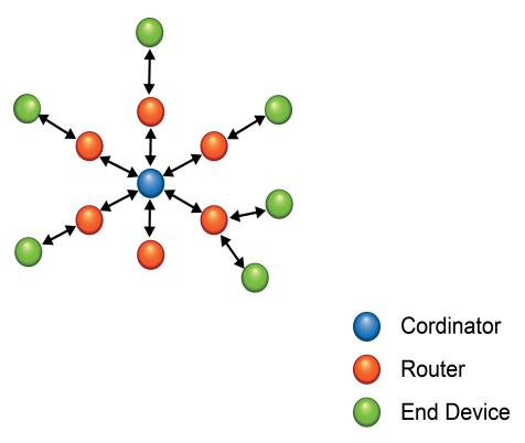
Each node that transmits the broadcast also creates an entry in a local broadcast transmission table. This entry to keeps track of each received broadcast packet to ensure the packets are not transmitted endlessly. Each entry persists for 8 seconds, and the broadcast transmission table holds 8 entries, effectively limiting network broadcast transmissions to once per second.
