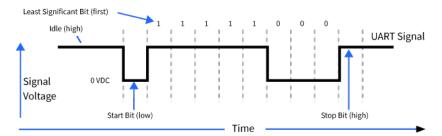
You can configure the UART baud rate, parity, and stop bits settings on the device with the **BD**, **NB**, and **SB** commands respectively. For more information, see Serial interfacing commands.
