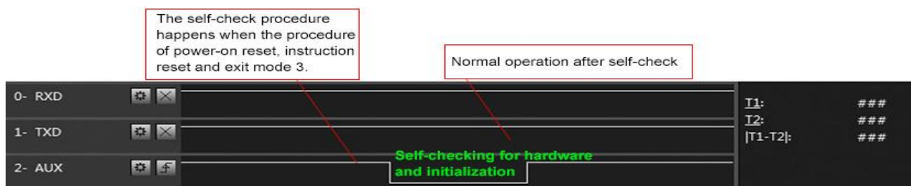
Timing Sequence Diagram of AUX when self-check
