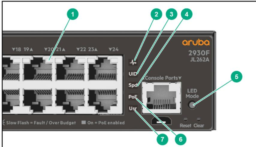
**Table 5:** Switch and port LEDs: Labels and description
