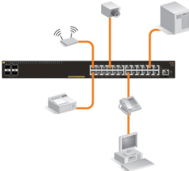
This illustration is an example of the switch being configured to supply PoE/PoE+ power to end devices such as IP telephones and wireless access points (WAPs).
