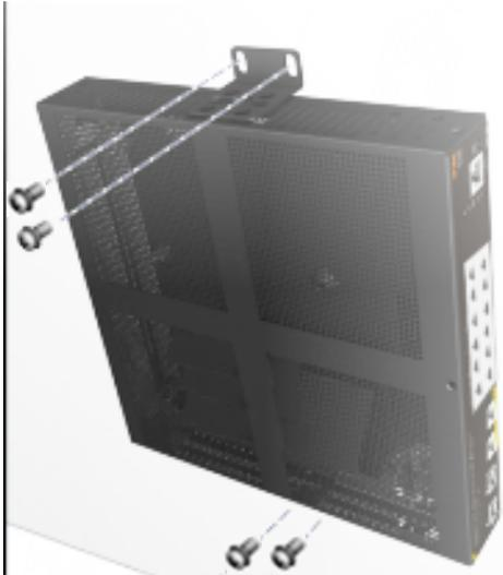
**Figure 27:** Wall mounting an Aruba 2930F 12G switch with ports facing downward
