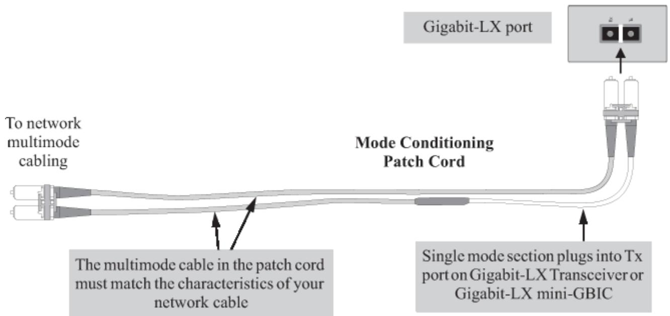
Be sure to purchase a patch cord that has appropriate connectors on each end, and has multimode fibers that match the characteristics of the multimode fiber in your network. Most important, the core diameter of the multimode patch cord must match the core diameter of the multimode cable infrastructure (either 50 or 62.5 microns).
