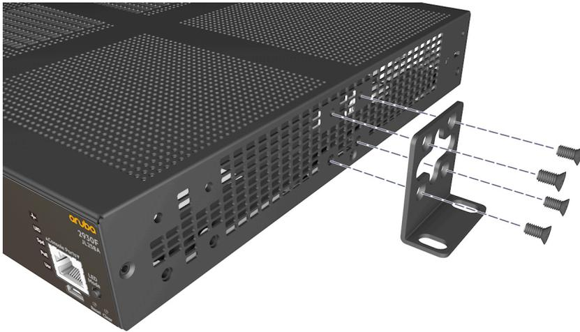
2. Attach the switch to the wall or under-table location using four 5/8-inch number 12 wood screws (not included).
