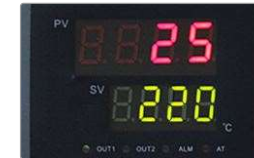
Using PID(Micro-computer) Temperature Control System
