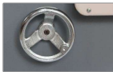
• Cutterbed Handwheel The lifting wheel adjusts the height of the cutterbed and controls the cutting length.
