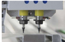
Dual Mounting Heads 360 Degrees Rotate by Any Angles
