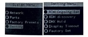
4-2) Press the "~" key, select "RDM Ongoing Set", then press the "Enter" key to execute the real-time RDM device search function.
