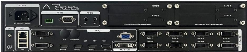
»» **Power Connector:** IEC standard power cable , input 100-240 VAC, 50 -60Hz.
