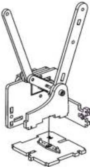
Step 28. Insert the Arm Bottom Plate into the Leh Arm Servo Plate at a diagonal angle and lever into place on the Pig Section.
