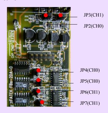
Please lookup the arrangement of jumper from the following table according to the desired output signal type.
